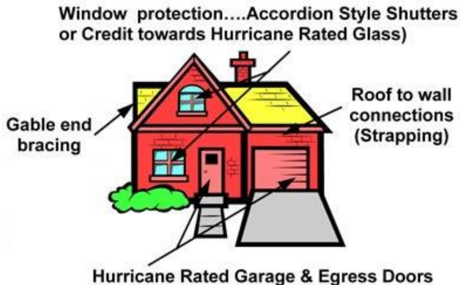
Figure 22. Illustrative example of a USA mitigation program that offers funding for upgrading ( http://retrofitswfla.org/ )
