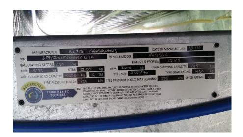
The load capacity of 345 kg was too low given that the caravan has 3 water tanks (2 x 90 litre washing and  $1 \times 60$  litre drinking; total of 240kg) and  $18 \times 60$  kg of gas. That leaves only 87 kgs for all other items listed above.
